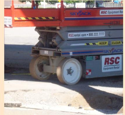
Scissor lifts could be driven into this hole and tip over.
