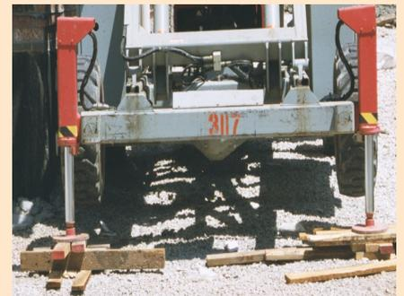
Unsafe: Blocking up scissor lifts outriggers with job site scrap.
