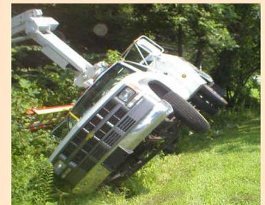
Set up to protect the truck from being struck by vehicles. Set up on stable and level ground.
