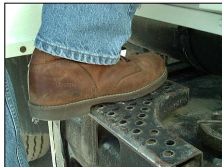
Facing the truck means better foot contact with steps and platforms.
